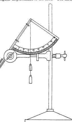
to such an angle that the meniscus at the lower end changes to a plane surface. The point at which this occurs is observed by the use of a pocket magnifier. This adjustment should be made in a good light with a sheet of white paper as a background. The angle A is then read and checked by readjusting 2 or 3 times and the length L of the liquid thread measured to 0.1 mm.
